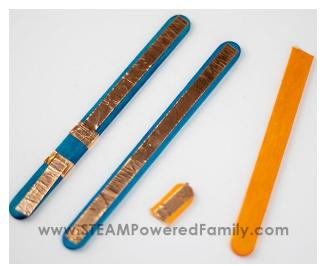
On the other outer craft stick run a strip of copper tape along the entire length. Here is a picture of all the sticks with copper tape, we will get to the little piece in a moment!
